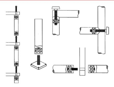
Inside Tube Diameter = 34.8-36.1Outer tube diameter = 1 1/2" Thread = M 10
